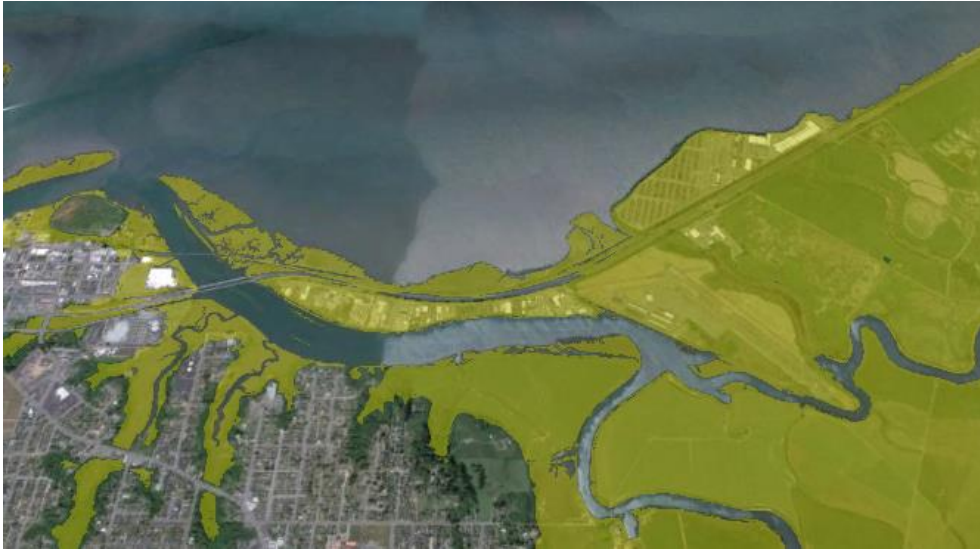
Figure 1: Freshwater Slough in Northern Eureka, CA. Inundation maps were developed by Jeff Anderson of Northern Hydrology & Engineering for the Humboldt Bay Sea Level Rise Vulnerability Assessment Project. The maps show areas vulnerable to existing and future sea levels that are currently protected from inundation due to the natural shoreline, dikes or berms, and railroad or road grades (Humboldt Bay Keeper 2017).
