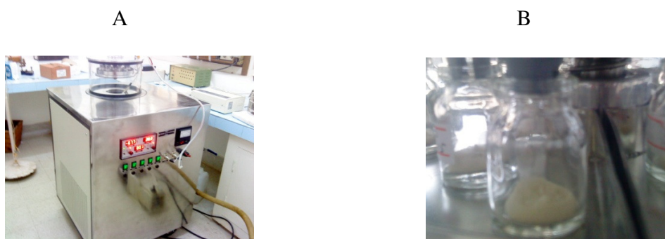
Figure 3: A) freeze drying system under operation, B) the diphyllin as lyophilized powder.
