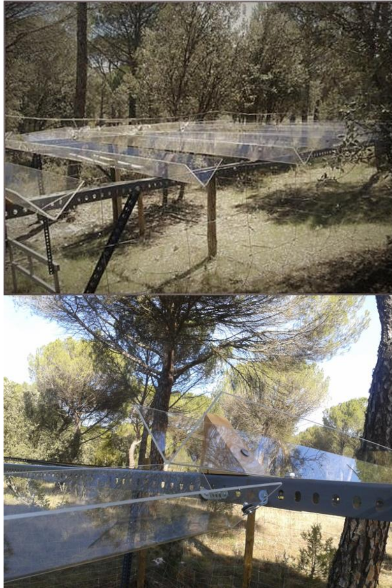
Fig. 4.2. Rain exclusion shelters formed by a metal frame supporting V-shaped clear methacrylate bands without UV filter.
