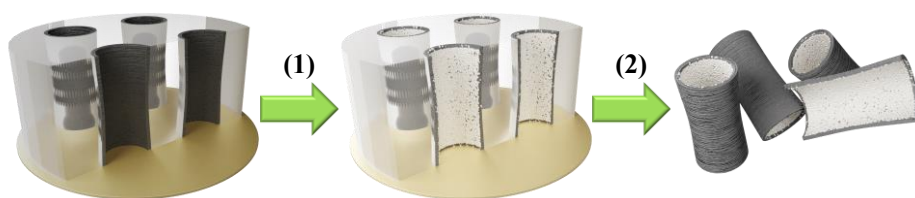
Figure 1. Electrodeposition of GPH/PtNPs micromotors. (1) Electrodeposition of outer sensing layer (GPH) and inner catalytic layer (PtNPs). (2) Micromotors release: polishing of sputtered gold layer and dissolving the polycarbonate membrane.
