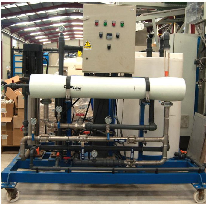
Fig. 12. Pilot membrane performance characterization system.
