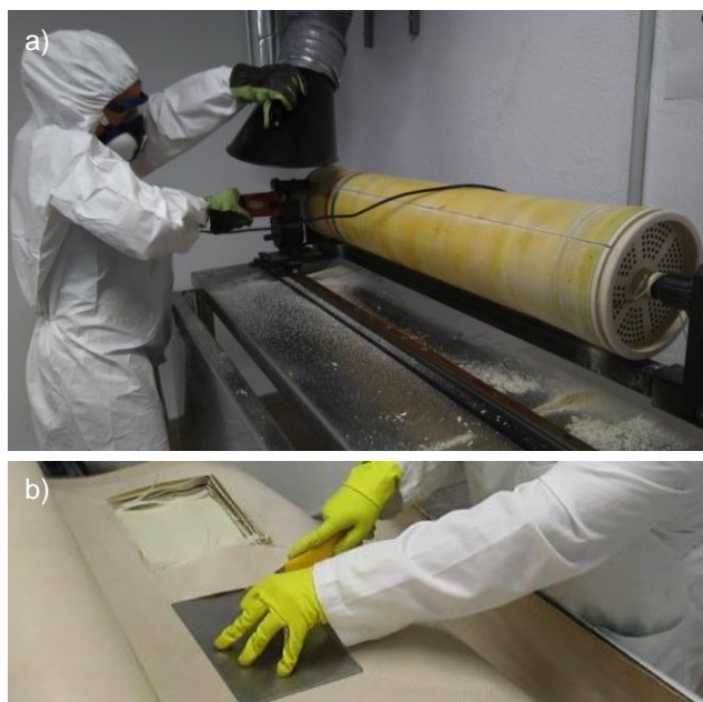
Fig. 8. End-of-life RO membrane autopsy: a) dissection of membrane module; b) extraction of membranes coupons.
