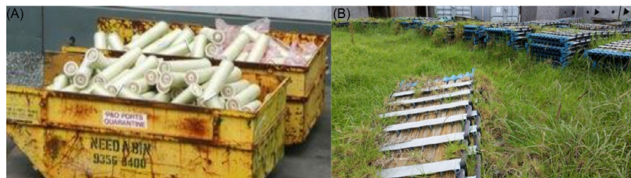
Fig. 5 End-of-life membranes collected in a shipping container in a desalination plant. Pictures by (A) Neil Palmer, reproduced with authorization and (B) Pierre Le-Clech.
