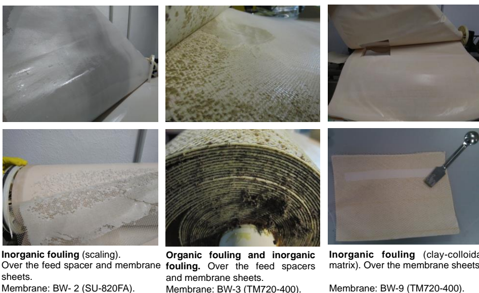
Fig. 13. Inorganic scaling (left), organic fouling (middle) and inorganic clay fouling (right) from different membranes installed in Spanish BWRO desalination plants (Paper II © Elsevier).
