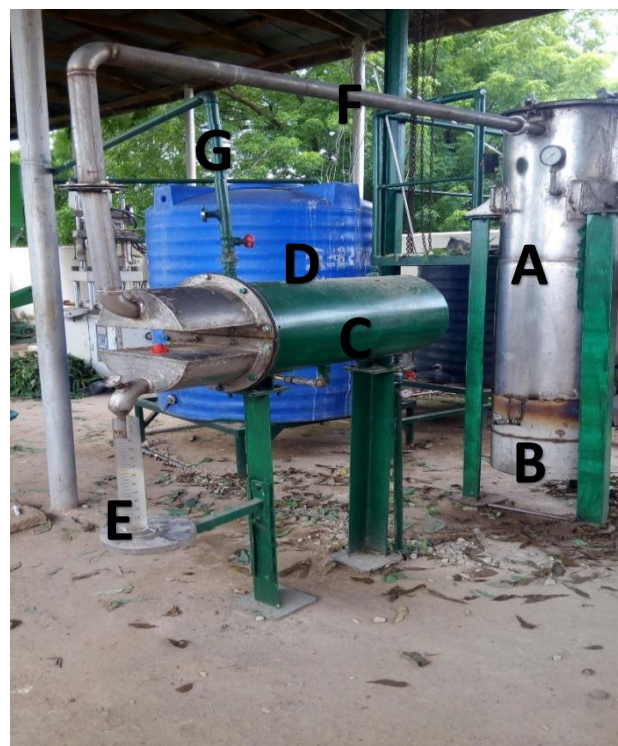
Figure 4: Steam distillation pilot plant for extracting essential oil from eucalyptus leaves
