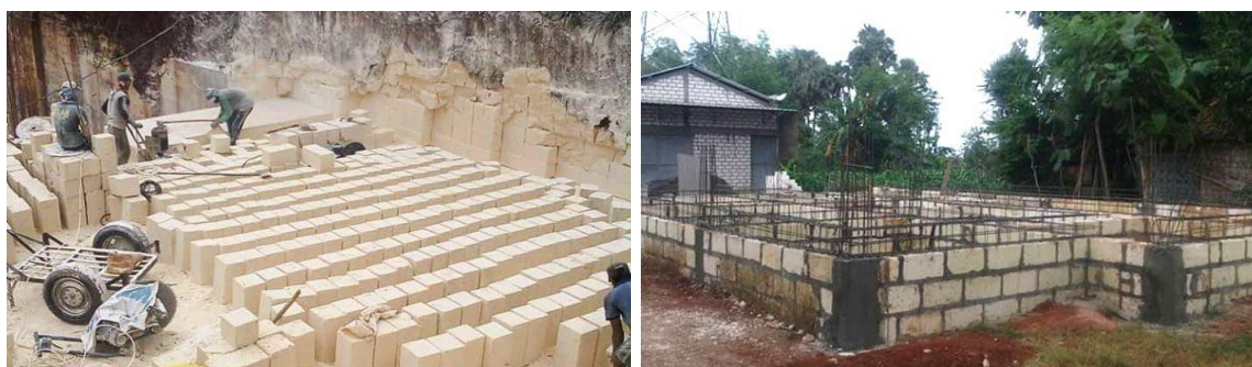
Figure 1. Processing of kumbang limestone as as building bricks in Rengel district, Tuban Regency (Source: left: https://lapak-properti.com/ ; right: https://batukumbongtuban.com/ )
