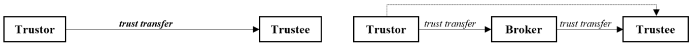
Figure 1: An illustration of two trust mechanisms from trustor to trustee . (Left: trust transfer mechanism with two involved parties; right: trust mechanism with three involved parties.)
