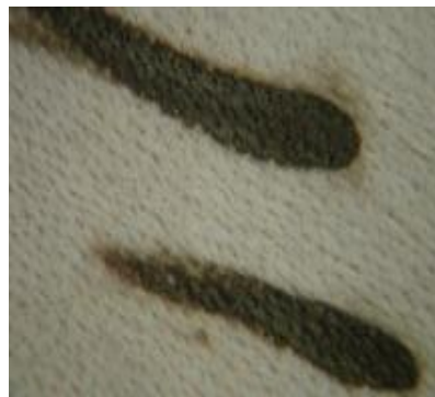
Staining in Staining with a run-off appearance concentrated spots A-Nickle-sulphide stains
