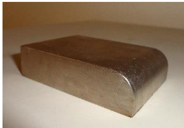
Figure 3. Steel rounded broad crested weir
