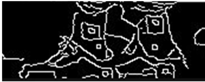
Figure 2.4: Canny Edge Implementation. Canny edge detection helps to visualize the edges of each feature so the user can easily find the shoe markers.
