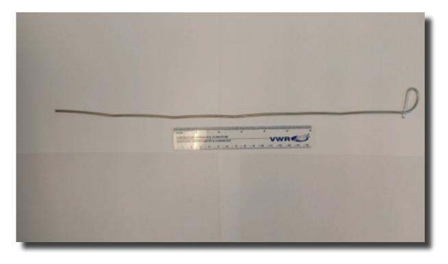
**STEP 5** – For each shellstring, string 12 of the drilled, cleaned shells onto a wire with the smooth (cupped) side down toward the bottom hoop. Bend the wire that is not covered by shell in half to provide a "handle" for hanging. Each string should take approximately 8-10 minutes in total to assemble.
