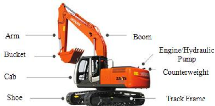
Figure 6.2. Parts of a Hydraulic Excavator (Hitachi, 2010).
