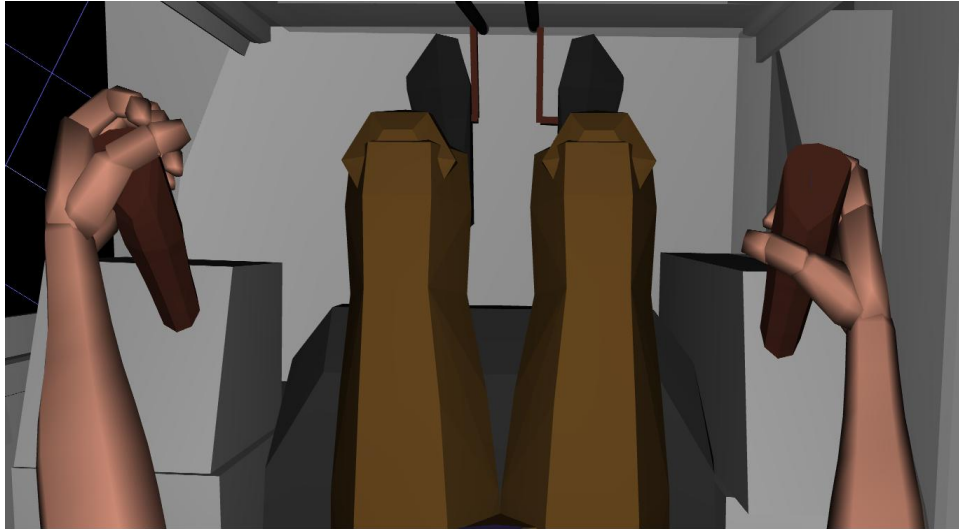
Figure B.1. Digital Human Model for Hydraulic Control Excavator System.
