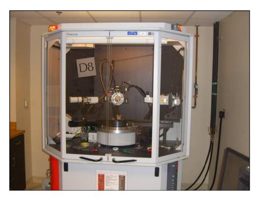
Figure 3.5. Bruker AXS D8 Discover XRD machine at NCAT.
