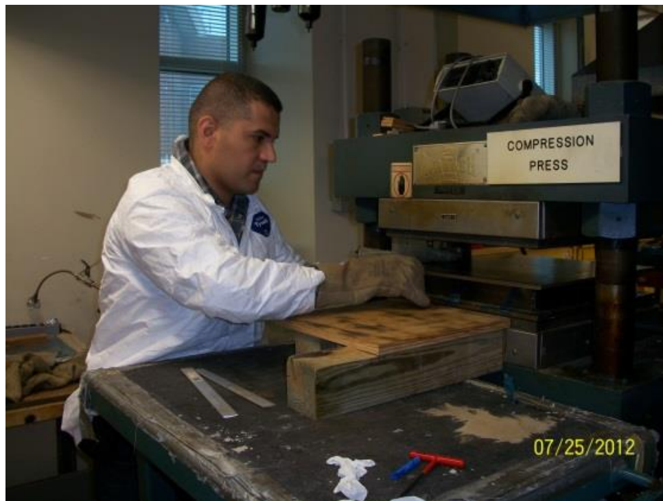
Figure 2.4. Photograph of preheating of mold and Eco-Core mixture.
