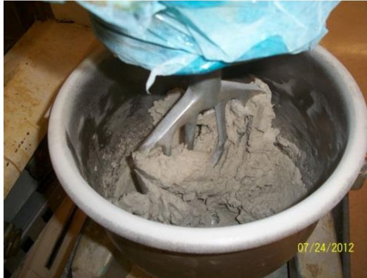
Figure 2.2. Fly ash-resin mixing process.
