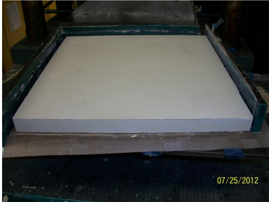
Figure 2.5. Photograph of cured Eco-Core panel.
