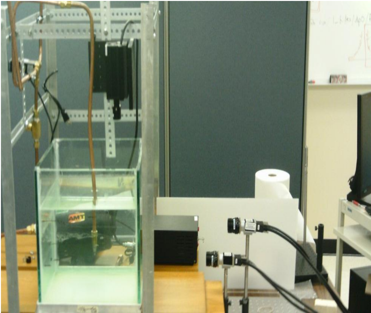
Figure 3.28. PIV setup, including the jet mixing tank.
