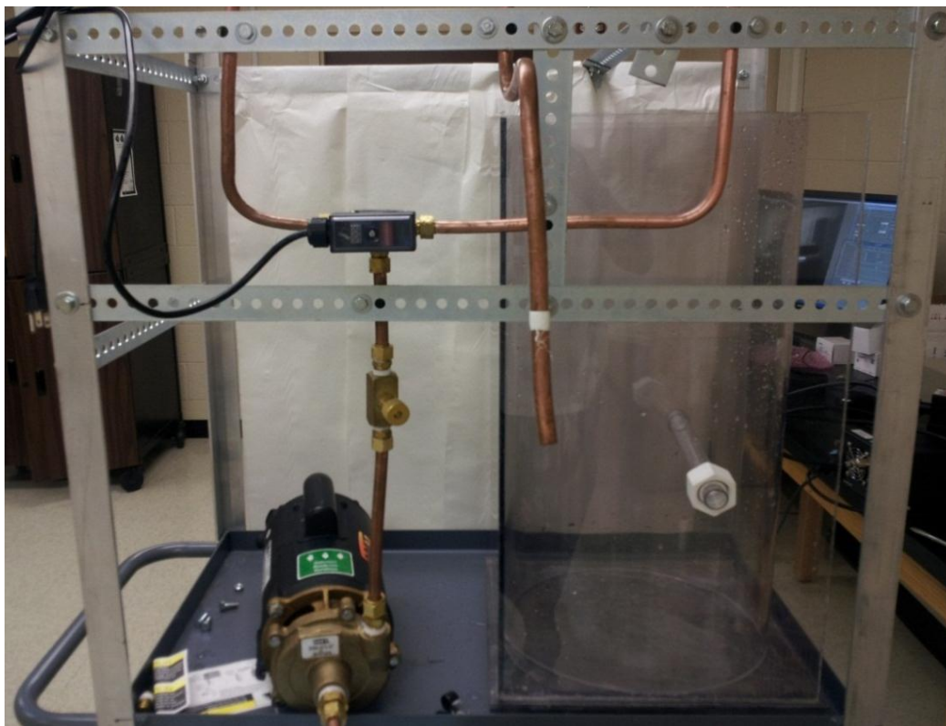
Figure 3.3. Actual jet mixing tank apparatus assembled on an aluminum cart.
