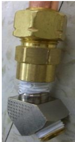
Figure 3.9. Actual jet nozzle using 45 degree elbow and recessed orifice plug.
