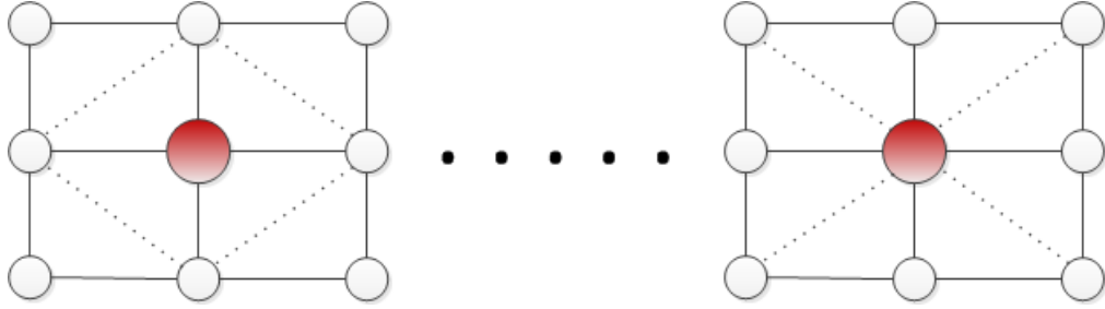
Figure 6.3. Clustering index: node has (a) four and (b) eight triangles incident on it.
