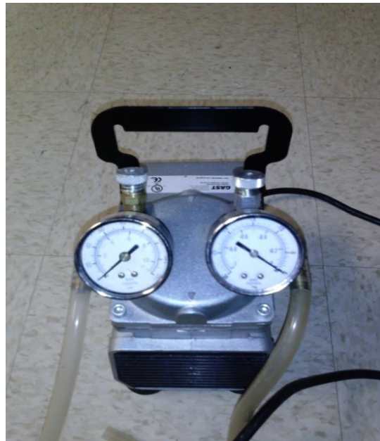
Figure 45. Vacuum pump for charging system
