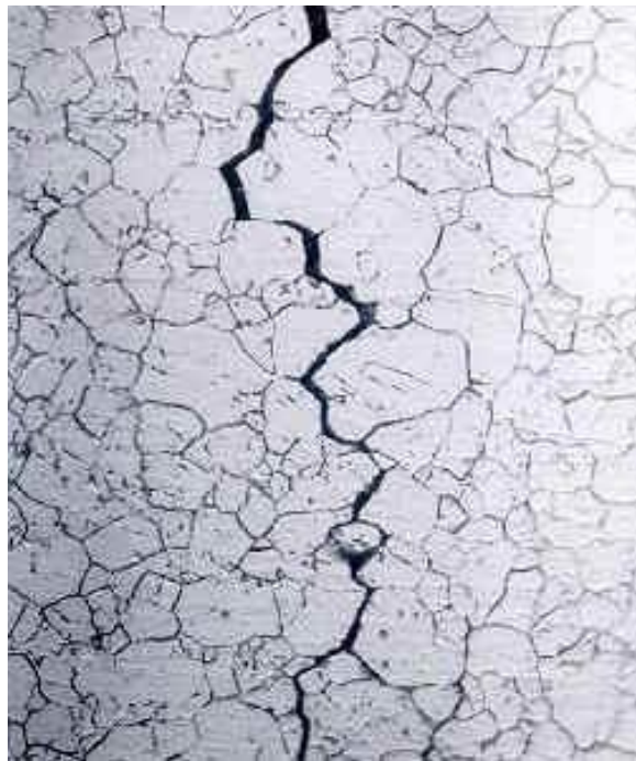
Figure 2.6. Intergranular stress corrosion crack. The crack follows the grain boundaries (Metallurgical Technologies 2012).
