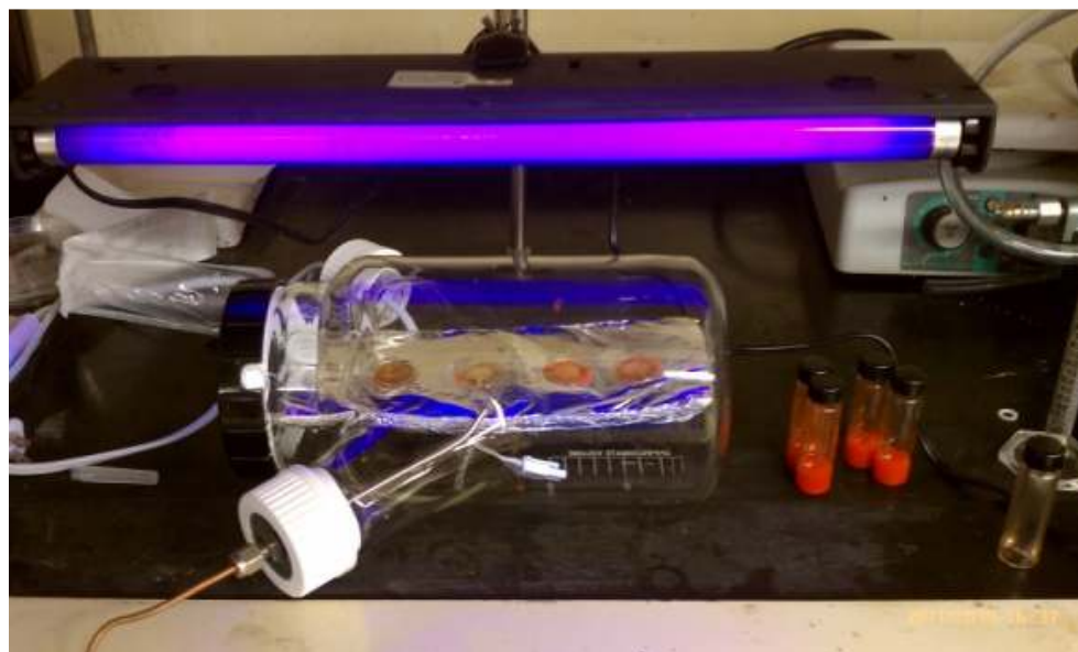
Figure 3.7. Polymerization of thin MIP film on QCM crystals inside photoreactor with nitrogen gas flow.
