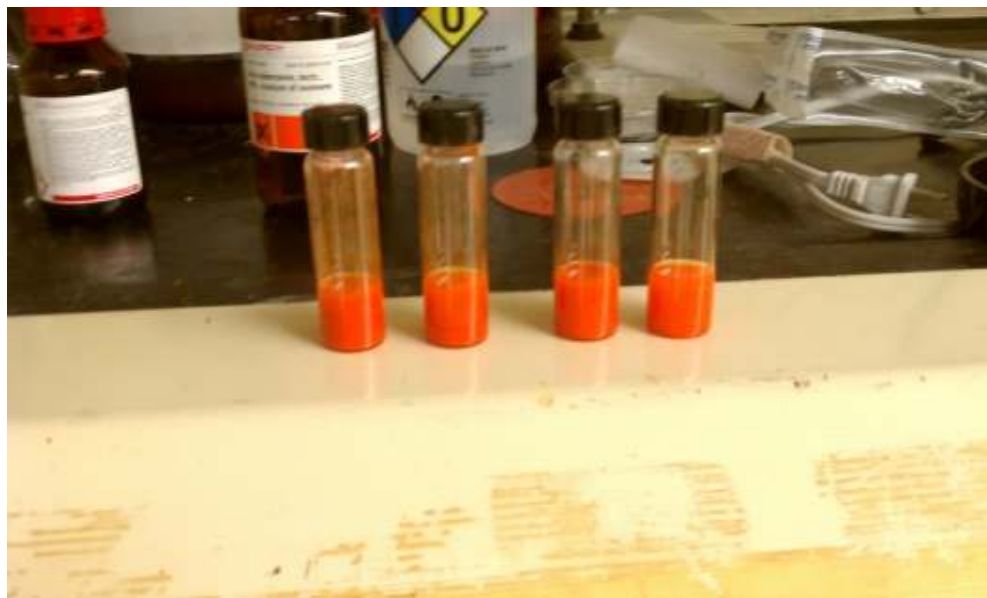
Figure 3.6. Prepolymerization solutions showing various template to monomer ratios
