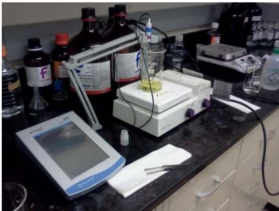
Figure 3.9. Setup for altering pH of bilirubin solution
