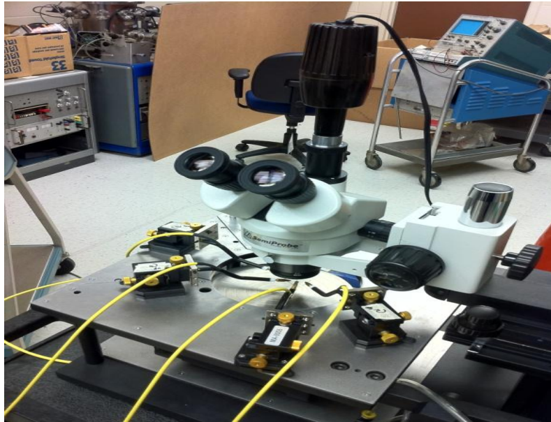
Figure 3.4. Four probe set up
