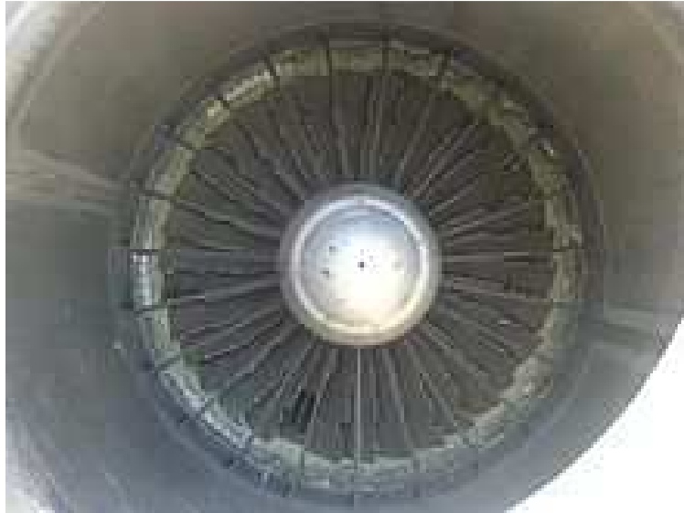
Figure 1.1. View of fan blades of JT8D jet engine after a bird strike [2]
