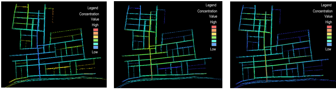
Fig. 5. (a) The concentration of mean depth; (b) The concentration of integration; (c) The concentration of connectivity
