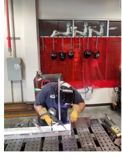
Figure 20: Welding Components to Sub Frame
