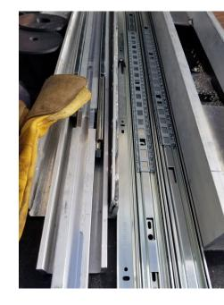
Figure 21: Disassemble of Linear Bearings
