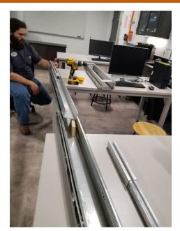
Figure 22: Marking the location of Linear Bearings
