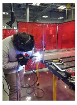
Figure 23: Welding of the Manufactured Hinges
