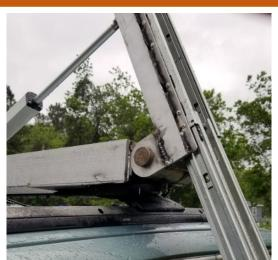
Figure 12: Hinge welded into subframe
