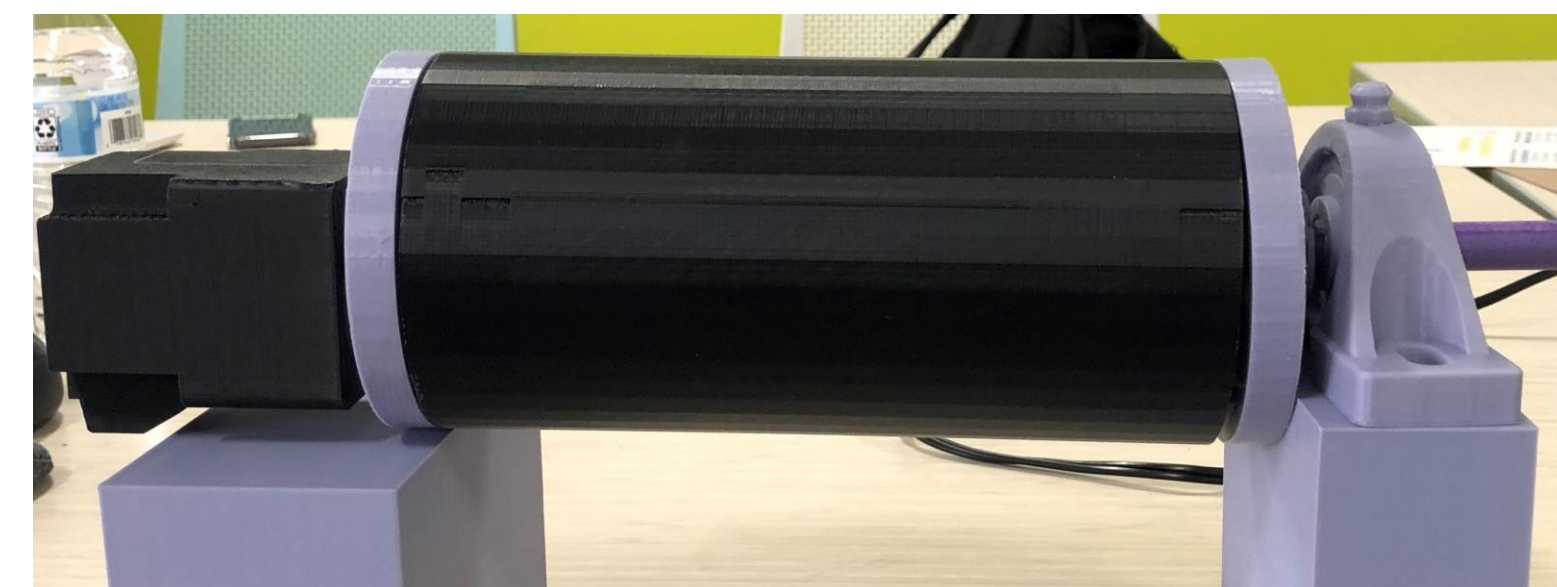
Figure 3: Many off-the-shelf parts were incorporated, and 3D printed. Shown is the speed-controlled motor, drum, interconnects, shaft, bearings and stands.
