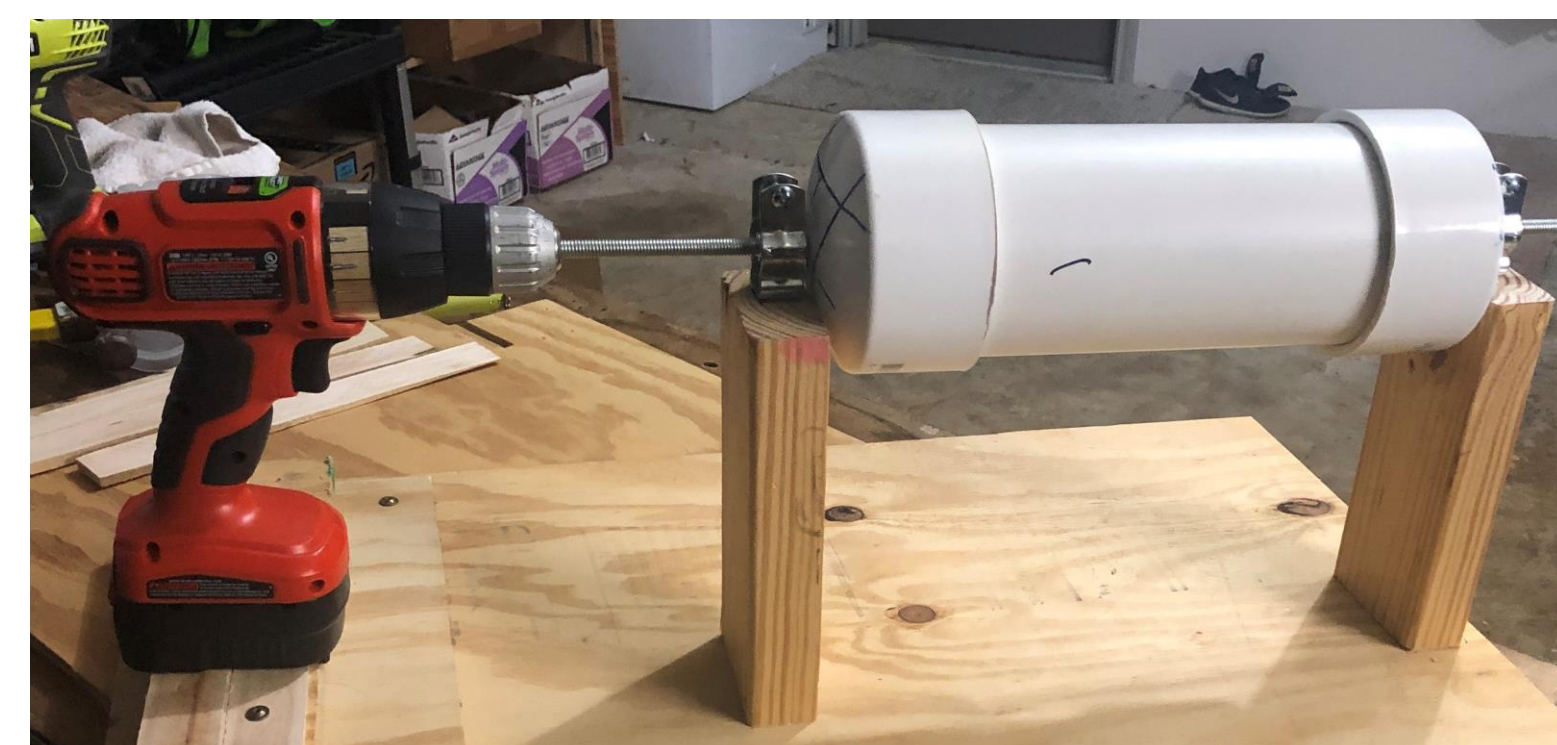
Figure 1: First mechanical prototype of a rotating collector drum using PVC pipe
