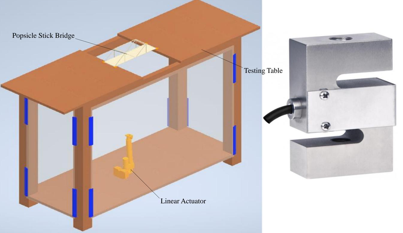
**Figure 2**: Linear actuator, general design of proposed device, s-type load cell
