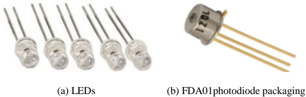
Figure 7: Type of the components used as a NIR pair.
