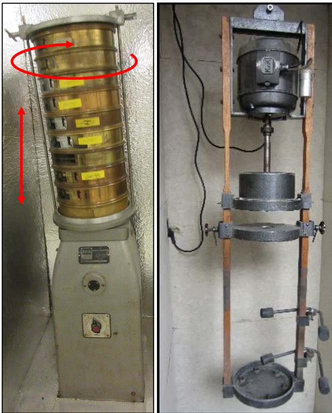
Figure 27: Sieving should be performed with a certified set of calibrated sieves, and by use of a sieving machine. At the left is the standard Pascall Inclyno model used at the Department of Geoscience. At the right is a custom-built version, suspended from the ceiling (seen at VIA University College in Horsens).
