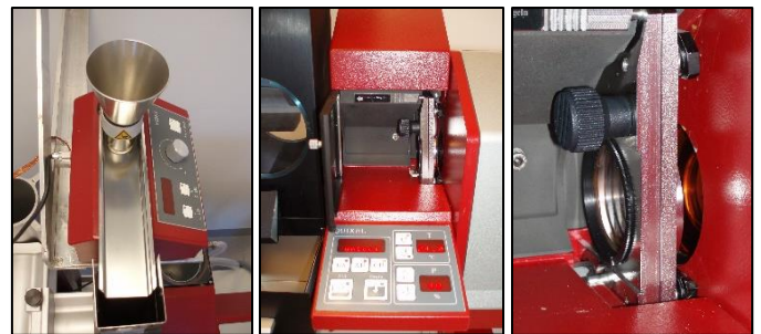
Figure 35: Different parts of the HELOS instrument, from left to right: VIBRI module (located above the GRADIS shaft), the QUIXEL module and the 2 mm flow-cell (which is inserted in the measuring area inside the QUIXEL module).
