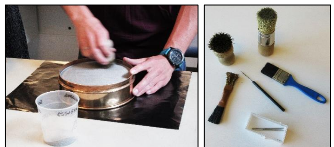
Figure 26: Use appropriate accessories to clean each sieve by hand (left), ranging from brushes of different material and sizes to various needles (right).
