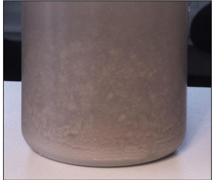
Figure 19: A flask containing material <0.063 \text{ mm} with visible flocs.
