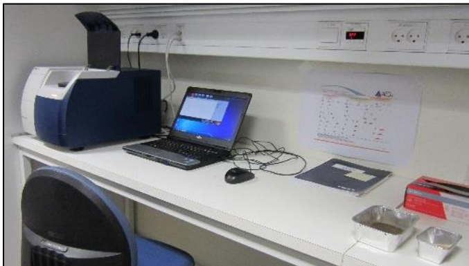
Figure 95: The Foss NIR table-top model as seen at Department of Agroecology, Aarhus University.
