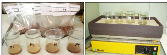
Figure 14: Oxidation process after 1 day (left) and from day 2 and onwards (right).
