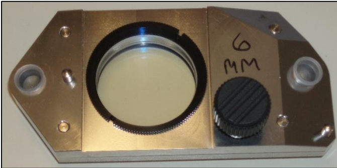
Figure 39: The 6 mm flow-cell.
