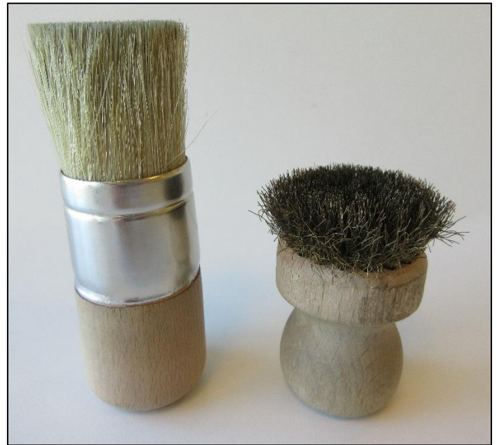
Figure 22: Use appropriate brushes for cleaning sieve meshes: To the left a soft-haired brush for soft (normally fine) mesh material and to the right a wire brush for metal mesh material.
