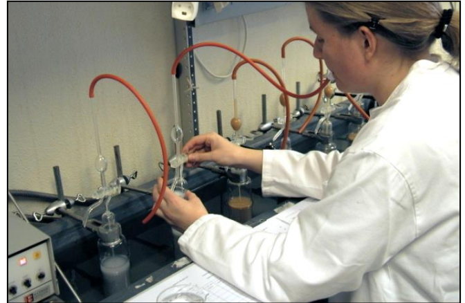
Figure 52: Sedimentation analysis with the Andreasen pipette method.
