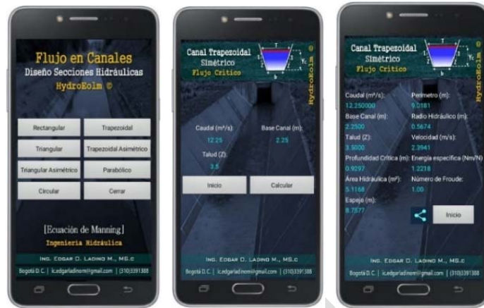
Figure 7. Trapezoidal channel, (Application solution for critical depth)
