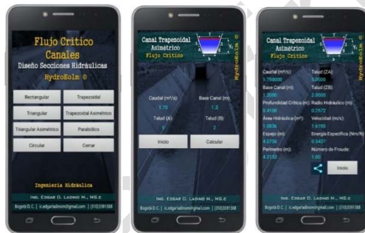
Figure 10. Asymmetric trapezoidal channel (Application critical depth solution)
