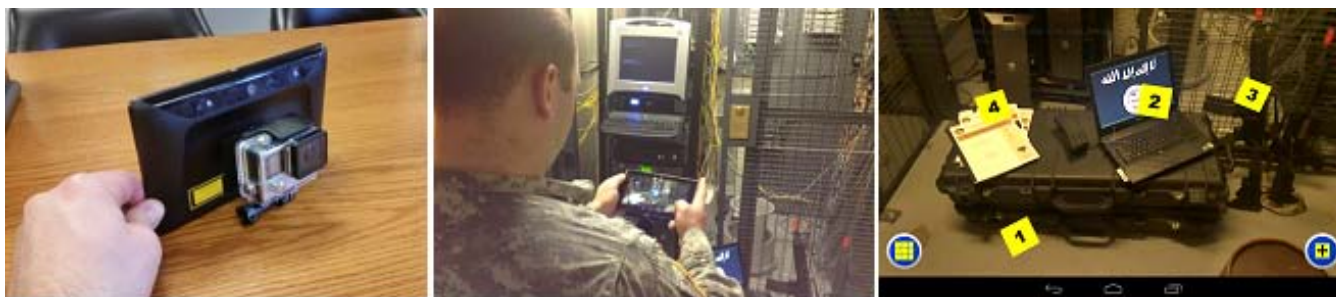
Figure 1. The Raven Eye system (left) is used by a soldier (center) to exploit a sensitive site. A screen capture from the system (right) shows tracked, virtual tags (yellow numbers) which annotate and geo-locate items of interest as the soldier navigates the scene.
