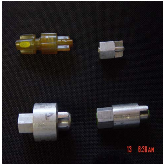
Figure 1. Flanged handles – bottom left, 6.4 mm; bottom right, (5.0 mm); top right (3.3 mm); top left (from medical device)
