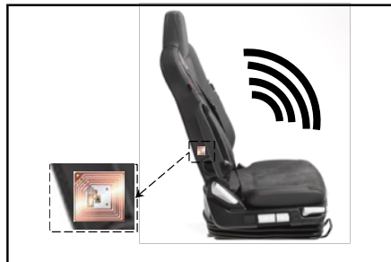
Figure 1. RFID-tagged automotive seat (Image sources: www.auroran.de , www.chriscdesign.co.uk )
