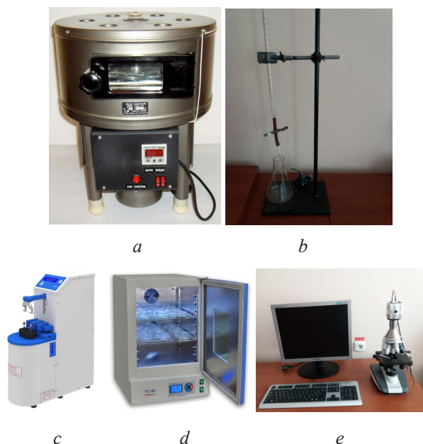
Fig. 2. Instruments and equipment used to determine the quality of flour and sourdough: a – drying cabinet SESH-3M; b – manual titration installation; c – PChP-3 device; d – dry-air thermostat TC-80; e – biological microscope XS-5510 MICRoMed
