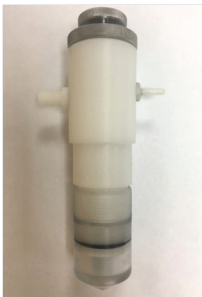
Fig. 2. Photographic representation of industrial sample of head for capsulation “through air”
