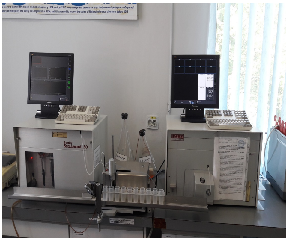
Fig. 1. device for determination of somatic cells «Bentley Somacount 150» (on the left) and for determination of physical-chemical composition of goat milk «Bentley Instrumentis» (on the right) (USA)
