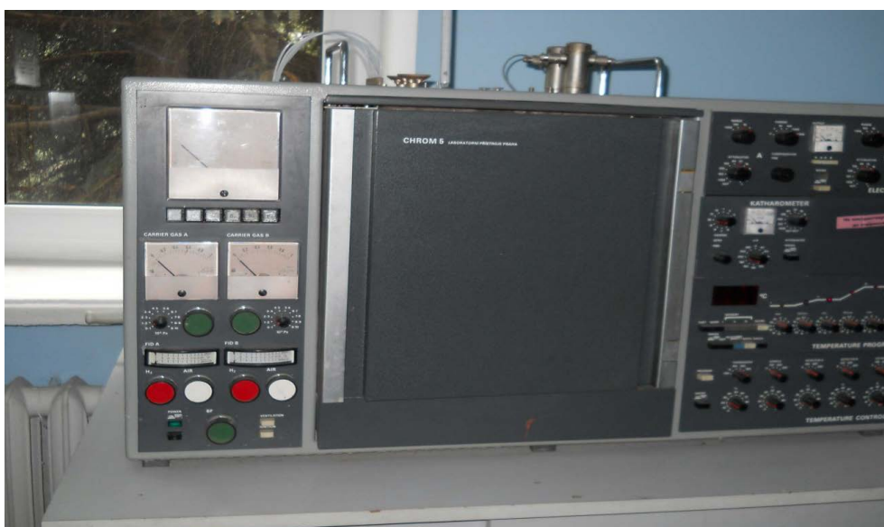
Fig. 3. Device chromatograph “Chrom-5» for determination of fatty-acid composition of the control and development batches of sour cottage cheese of goat milk (USA)
