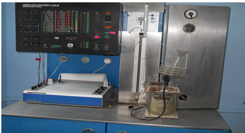
Fig. 2. Device for determination of the amino acid composition of the control and development batches of cottage cheese of goat milk – automatic analyzer of amino acids AAA 339 M (Prague)
