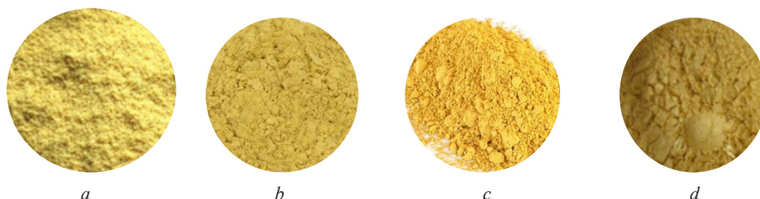
Fig. 2. Samples of bee pollen of different dispersity degrees: a – 115 \pm 5 mcm; b – 20 \pm 2 mcm; c – 15 \pm 2 mcm; d – 10 \pm 2 mcm
