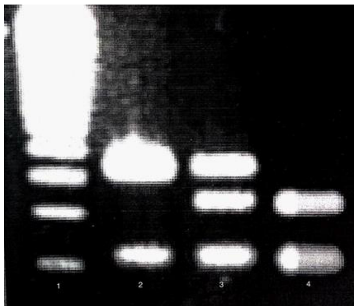
Fig. 1. Electrophoregram of human DNA samples containing the 105Ile/Val polymorphism of the GSTP1 gene: 1 – molecular steps; 2 – homozygote 105Ile/Ile; 3 – heterozygote 105Ile/Val; 4 – homozygote 105Val/Val.
