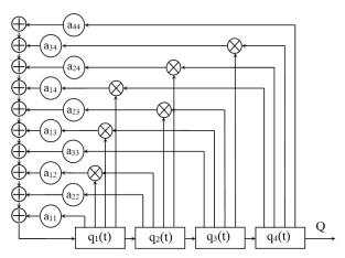
Fig. 1. General NLFSR construction
