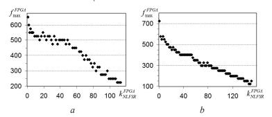
**Fig. 4.** Dependence of  $f_{\text{max}}^{\text{FPGA}}$  on  $k_{\text{NLFSR}}^{\text{FPGA}}$ : a – for L = 28, b – for L = 29
