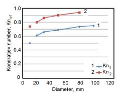
Fig. 2. Effective Kondratjev number Kn versus diameter of cylindrical probes made of AISI 304 steel when quenching in 8 % water solution of NaNO<sub>3</sub> at 20 °C: 1 – quenching in still solution; 2 – quenching in solution flow 1.5 m/s
