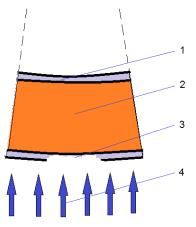
**Fig. 4.** A scheme explaining why a big distortion takes place during quenching in water PAG polymers solutions: 1 – polymer coating; 2 – quenched steel part; 3 – locally dissolved by water flow polymer coating; 4 – water flow
