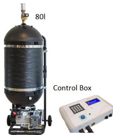
Figure 7 PULSE-80 and associated control box (NC test)
