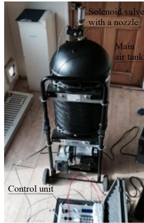
Figure 15 Setup of PULSE-80 unit
