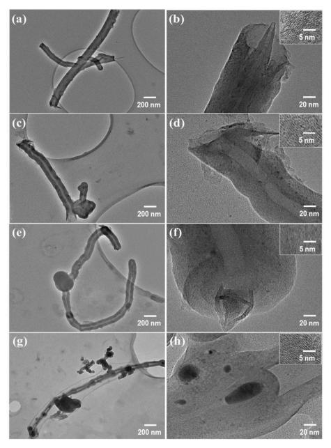
Fig. 2. TEM micrographs of the CNT reinforced foams. (a–b) CNT<sub>0.005\_0.5h</sub>; (c–d) CNT<sub>0.005\_1h</sub>; (e–f) CNT<sub>0.01\_0.5h</sub> and (g–h) CNT<sub>0.01\_1h</sub>. The inset shows the corresponding lattice fringe of the carbon structures.
