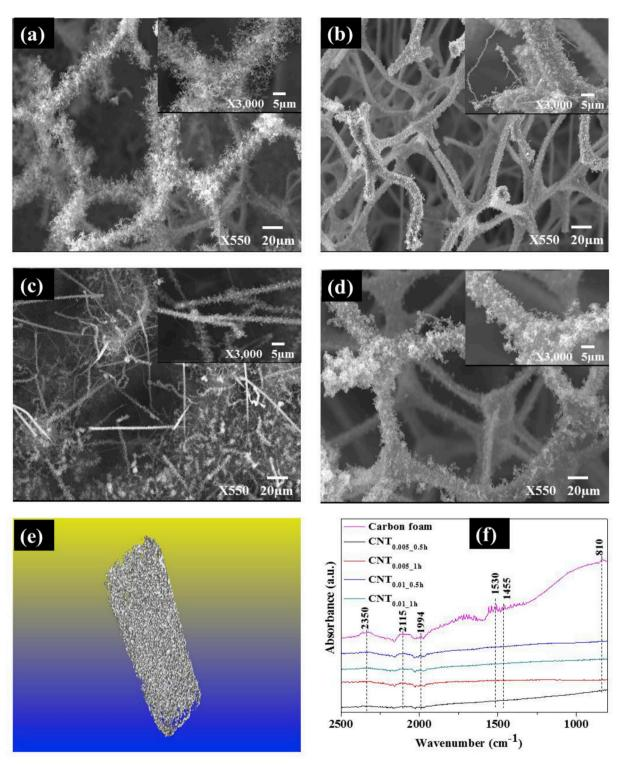
**Fig. 1.** Morphological and structural characteristics of the CNT-reinforced foams. (a) SEM micrograph of the  $CNT_{0.005_{.0.5h}}$  foam; (b) SEM micrograph of the  $CNT_{0.005_{.1h}}$  foam; (c) SEM micrograph of the  $CNT_{0.01_{.0.5h}}$  foam; (d) SEM micrograph of the  $CNT_{0.01_{.1h}}$  foam; (e) Micro-CT image of  $CNT_{0.01_{.1h}}$  foam; and (f) ATR-FTIR spectra of the CNT-reinforced foams synthesized at different mass concentrations of precursors and dwell time.
