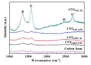
Fig. 3. Raman spectra of carbon and CNT-reinforced foams.
