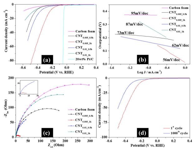
Fig. 5. (a) Polarization curves of 20 wt% Pt/C, carbon and CNT-reinforced foams in 0.5 M H<sub>2</sub>SO<sub>4</sub>, (b) Tafel plots, (c) Nyquist plots at 250 mV overpotential, and (d) HER polarization curve of CNT<sub>0.005,1h</sub> before and after 1000 cycles of CV in 0.5 M H<sub>2</sub>SO<sub>4</sub>.
