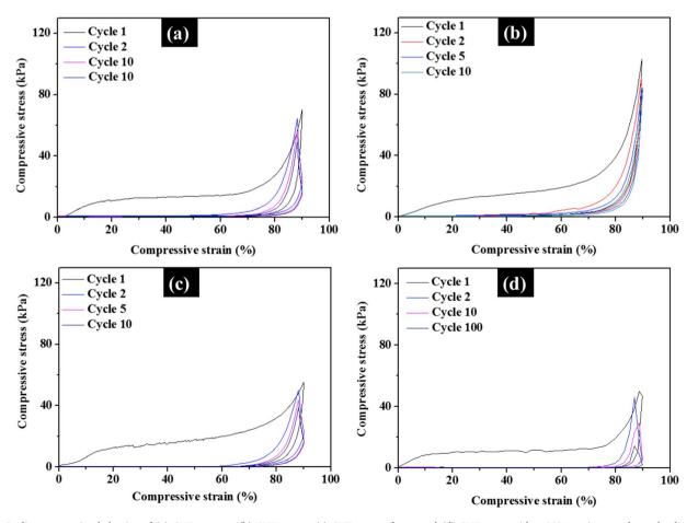
Fig. 4. Cyclic compressive behavior of (a)  $CNT_{0.005\_0.5h}$ ; (b)  $CNT_{0.005\_1h}$ ; (c)  $CNT_{0.01\_0.5h}$  foam; and (d)  $CNT_{0.01\_1h}$  with a 90% strain, tested at a loading rate of 8 mm/min.
