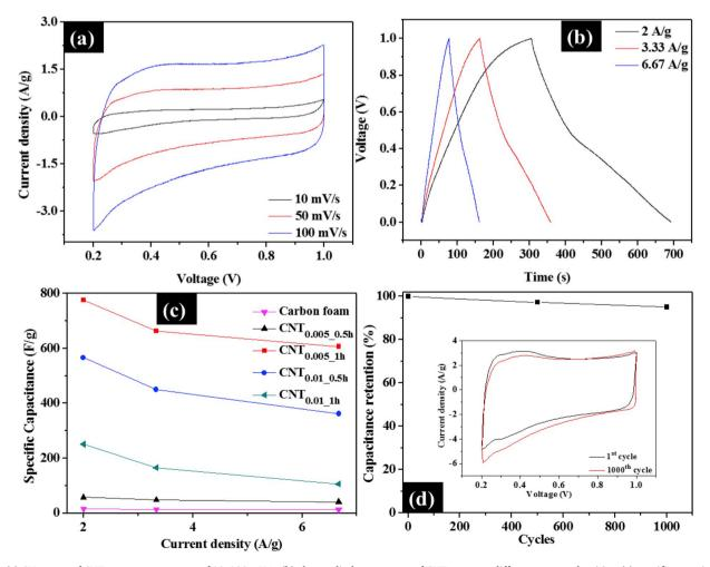
**Fig. 6.** (a) CV curves of CNT<sub>0.005\_1h</sub> at scan rates of 10–100 mV/s, (b) charge-discharge curves of CNT<sub>0.005\_1h</sub> at different current densities, (c) specific capacitance of the CNT-reinforced foams as a function of current density, in 0.5 M H<sub>2</sub>SO<sub>4</sub>, and (d) cycling performance of the CNT<sub>0.005\_1h</sub> foam at 1st and 1000th cycles, at 2 A g<sup>-1</sup>.
