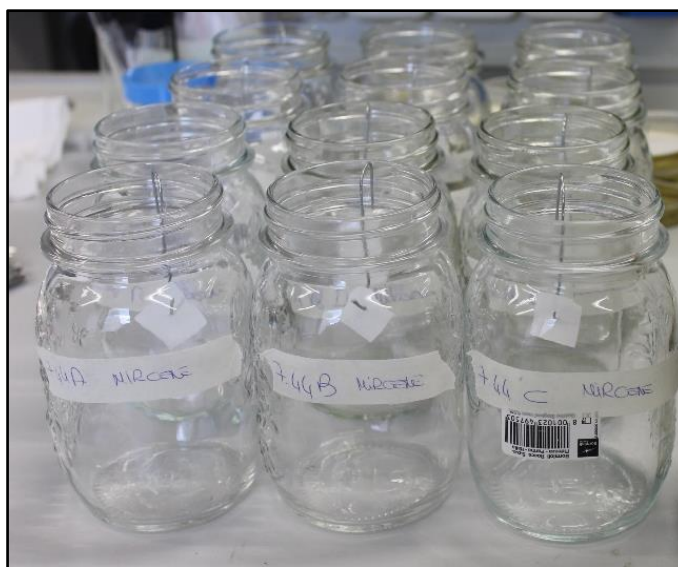
Figure 3.8. Glass container for fumigant bioassay
