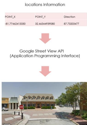
Figure 4 The process of getting geo-tagged images using Google Street View API
