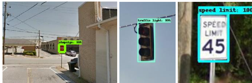
Figure 13 Types of detected traffic signs
