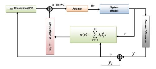
Figure 1: Block diagram of the sliding-PID controller
