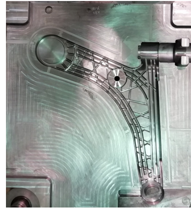
Figure 7. Mold of the suspension arm.
