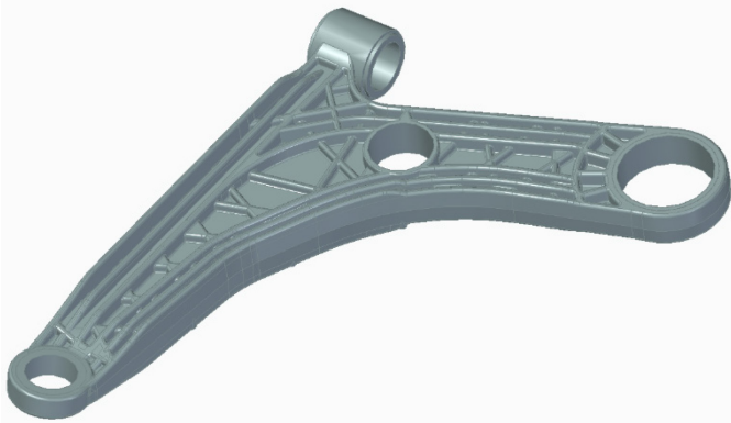
Figure 1. 3D model of the suspension arm.
