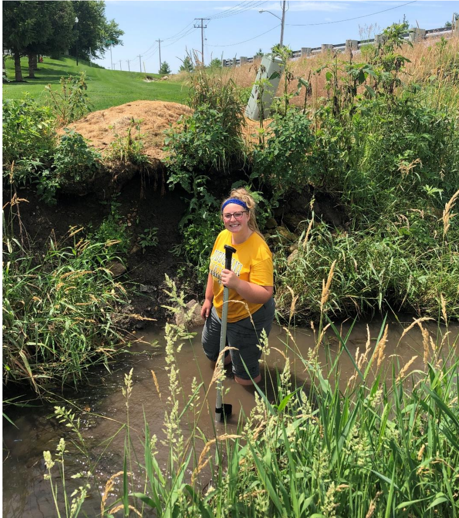
Figure 4: Researcher Morgan Anderson using flow meter to record the average velocity of Crow Creek.
