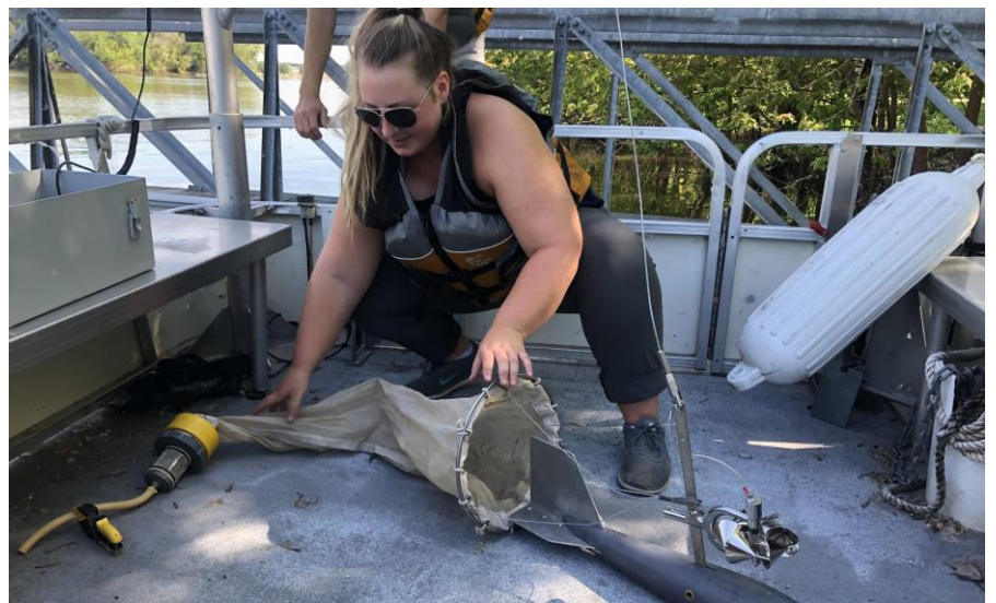
Figure 3: Researcher Morgan Anderson aboard Augustana's research boat The Stewardship with sampling net attached to a weight and flow meter by a suspended wire reel (Photo taken by Alex Disabato).
