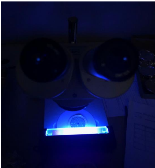
Figure 7: Dissecting microscope, filtered sample, and UV light used to identify plastic particles.
