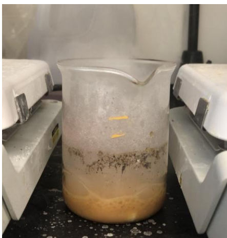
Figure 5: Hydrogen peroxide (30%) and iron (II) sulfate added to sieved sample in order to digest organic compounds.
