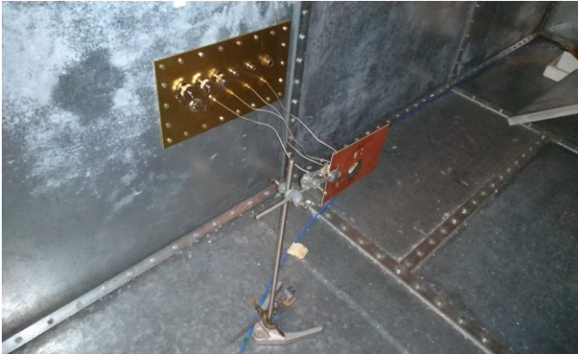
Fig. 2 Measurement Jig in the Reverberation Chamber.
