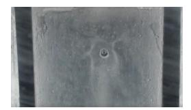
Fig. 4. 3: 300 s cleaning, 1 lmin<sup>-1</sup> jet, 0.19 mm WSP thickness, water temperature 20 °C.
