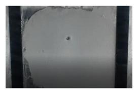
Fig. 4. 9: 300 s cleaning, 1 Imin<sup>-1</sup> jet, 1.9 mm WSP thickness, water temperature 20 °C.
