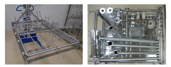
Fig. 3. 3: Left: Rack 1 unloaded. Each pipe section can be seen leading to a nozzle on to which a component is loaded. Right: Rack 1 with disassembled components loaded on to jet/spray nozzles (Rodgers et al. 2019).
