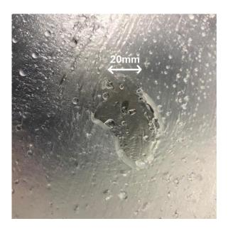
Fig. 5. 5: Cleaned area close-up after one hour of cleaning: 1 lmin<sup>-1</sup> spray, 0.19 mm WSP thickness, water temperature 20 °C, 50 mm standoff.
