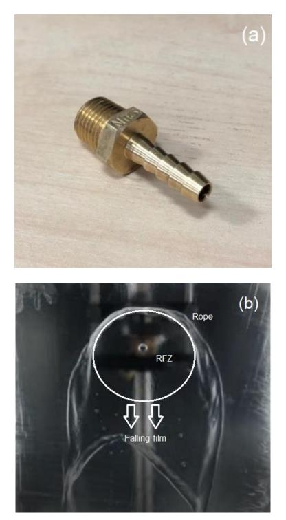
Fig. 3. 14: Top: Jet nozzle, bottom: footprint of horizontal 1 lmin<sup>-1</sup> jet impinging on vertical Perspex wall. Key regions observed by Wilson et al. (2018) highlighted: rope, RFZ and falling film
