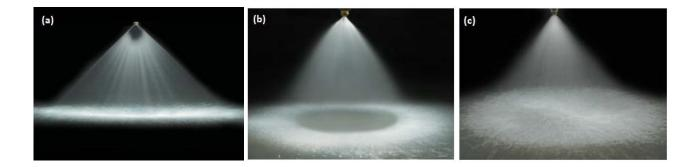
Fig. 2. 7: Spray distributions: a) Flat fan, b) Hollow cone, c) Full cone (PNR, Accessed: 27/2/19).
