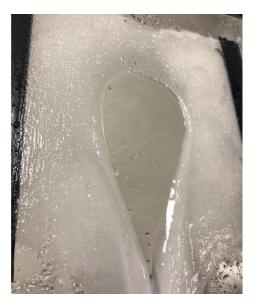
Fig. 5. 36: Long-time (300 s) clean area close up (1 Imin<sup>-1</sup> spray, 0.95 mm WSP thickness, water temperature 40 °C).
