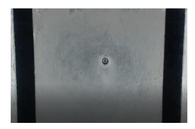
Fig. 4. 6: 300 s cleaning, 1 lmin<sup>-1</sup> jet, 0.95 mm WSP thickness, water temperature 20 °C.
