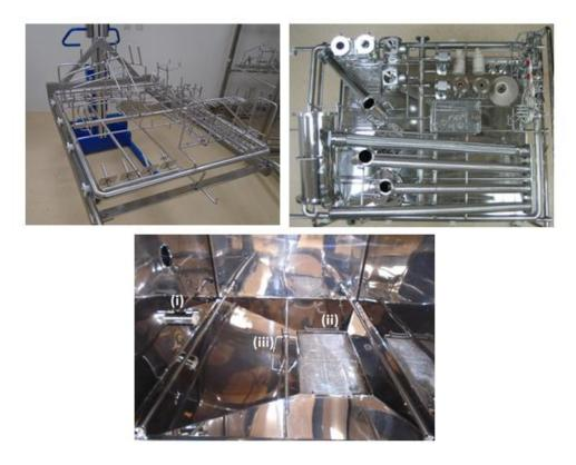
Fig. 2. 34: a) Wash rack unloaded. Each pipe section can be seen leading to a nozzle on to which a component is loaded (b) Wash rack with disassembled components loaded on to jet/spray nozzles (c) Wash rack is loaded into washer via coupling (i), water is recirculated via sump (ii) rinse of the chamber is performed by rotating jet arm (iii) (Rodgers et al., 2019).
