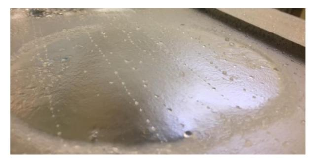
Fig. 5. 29: Cleaned area close-up after one hour of cleaning: 2.5 Imin<sup>-1</sup> spray, 0.19 mm WSP thickness, water temperature 20 °C, 125 mm standoff.
