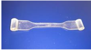
Fig. 9. The fatigue test specimen made from Tango Plus flx930.
