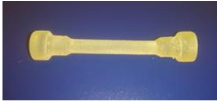
Fig. 5. The tensile test specimen made from Tango Plus flx930.
