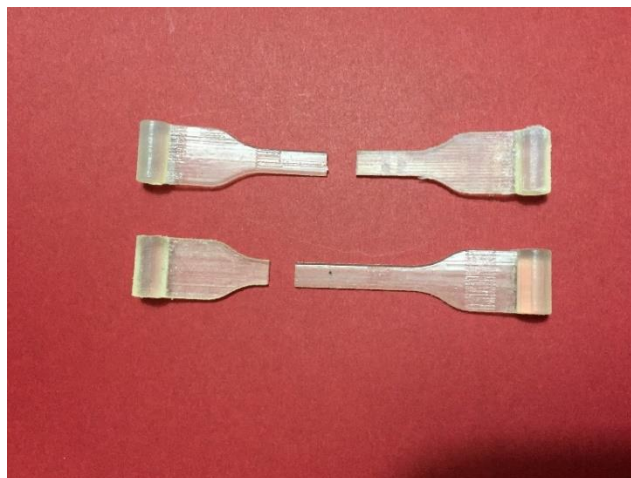
Figure 4.18 The fatigue test specimens made from Tango Plus after test.
