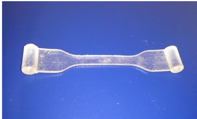
Figure 4.17 The fatigue test specimen made from Tango Plus.
