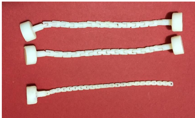
Figure 5.11 The 4.5 mm diameter 3D printed chains compared with the 3 mm diameter 3D printed chain.
