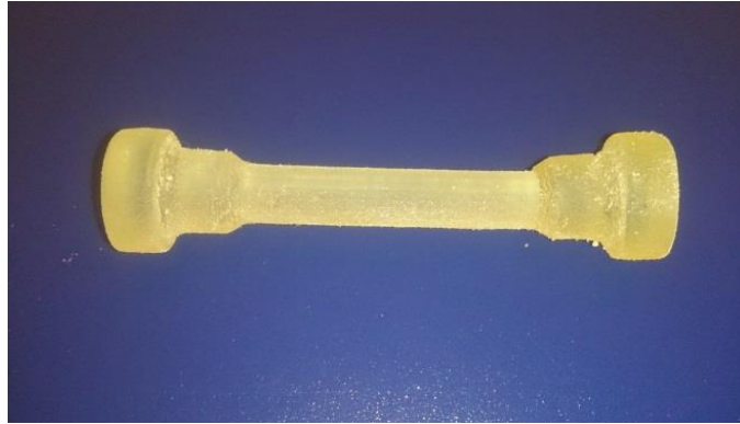
Figure 4.8 The tensile test specimen made from Tango Plus flx930.
