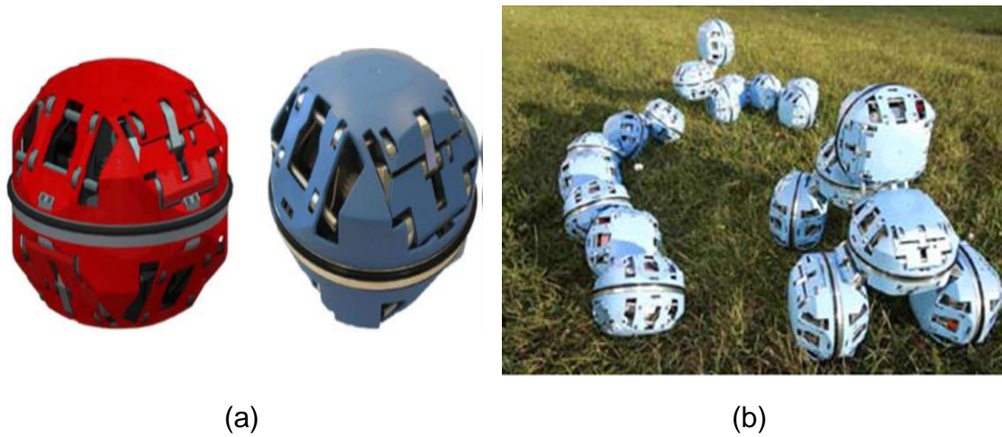
Figure 2.2 (a)The ATRON module, 11 cm in diameter. Left: CAD model of the ATRON module with plastic cover. Right: Photo of a fully functional ATRON. (b) Three groups of seven ATRON modules. From left to right, the configurations are snake, cluster-walk and car [18].
