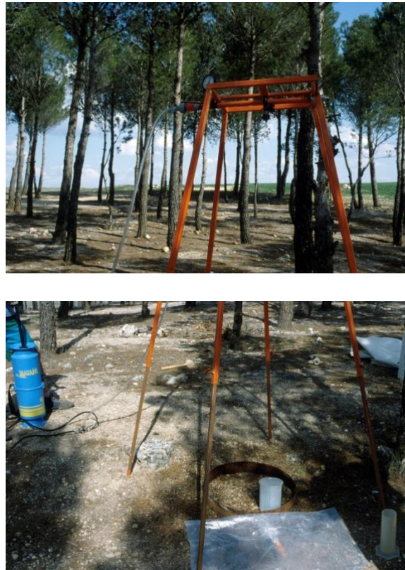
Figure 2.7: Portable rainfall simulator prior to experimentation without curtain.
